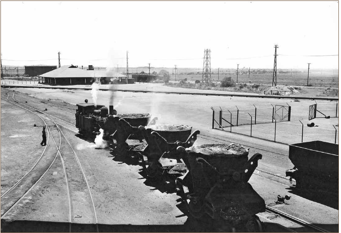
Top Right: Prior to standardisation of the steelworks, one of the 2-6-2 tank locomotives shunts three slag pot wagons at No. 1 blast furnace, Whyalla c.1960. BHP Archives.
