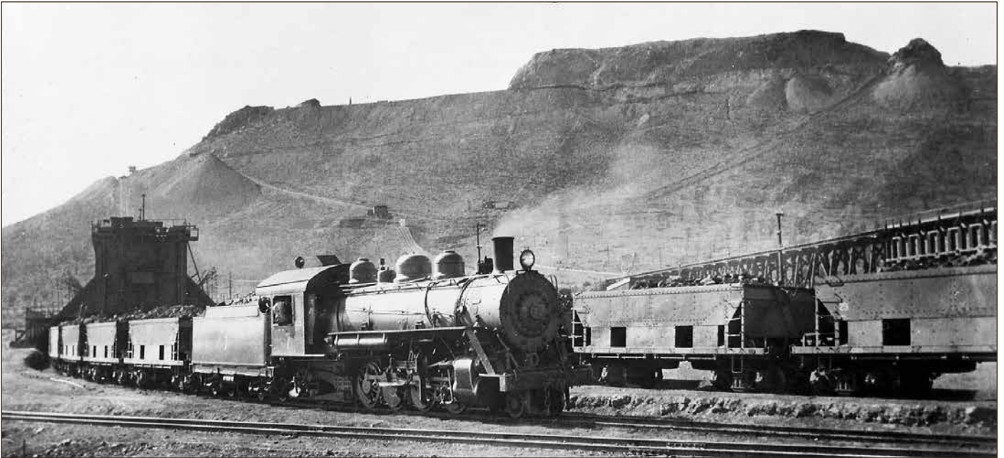
This 1934 scene of Iron Monarch and its bins shows Mikado No. 7 assisting to load 'D' class ore trucks. BHP Archives.
