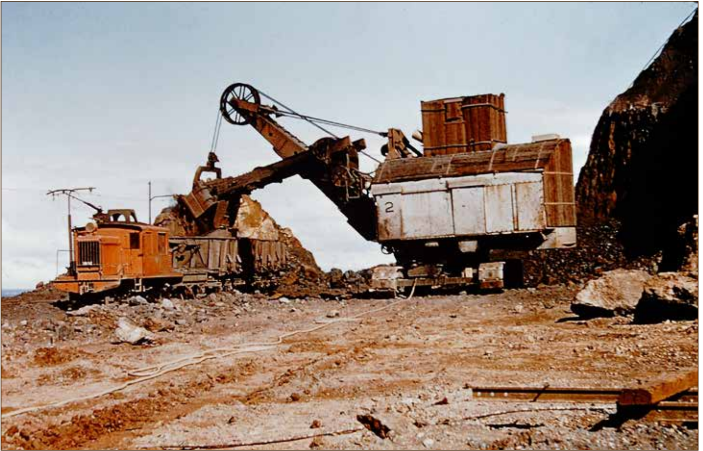
PE1, working as an electric locomotive, assists electric shovel No. 2 to load a quarry train in 'F' bench, Iron Monarch c.1956. BHP Archives.
