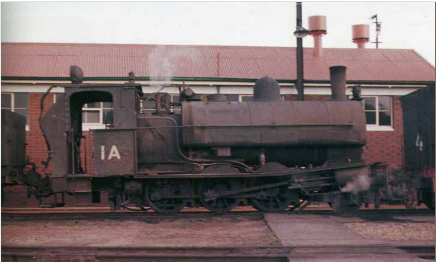
Its days are numbered! 2-6-0 ST No. 1A stands 'on shed' in the locomotive depot, Whyalla, in May 1962. BHP Archives.
