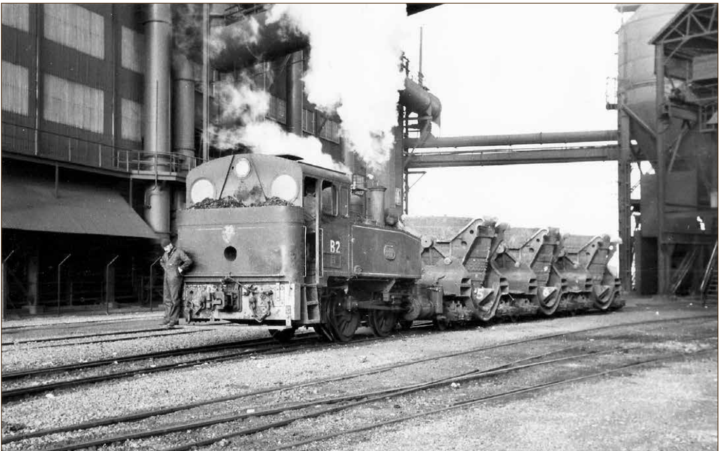
Ex-Newcastle steelworks standard gauge steam locomotive B2 hauls a rake of three hot metal ladle cars from the blast furnace at Whyalla during 1964. D. Worth.
